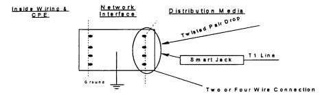
Figure 1 - Network Interface Device
