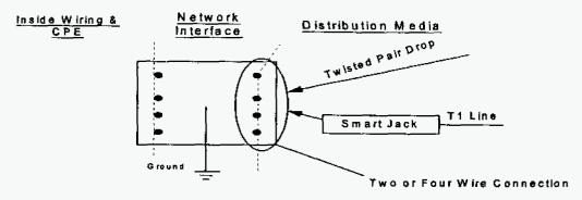
Figure 1 - Network Interface Device
