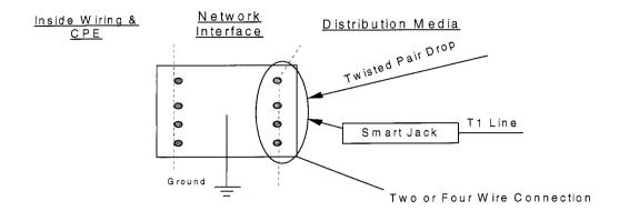
Figure 1 - Network Interface Device
