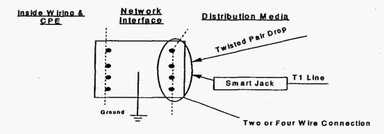
Figure 1 - Network Interface Device
