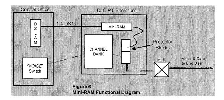
Connecting the Mini-RAM to the existing cable is accomplished through the use of a cable assembly specially designed for this application. The cable assembly plugs into the Mini-RAM connectors on one end and the other end fans out into 8 connections to allow the mini-RAM to be connected to any line served by the DLC in that enclosure. That connection is accomplished by removing the protector unit from the desired line at the protector
