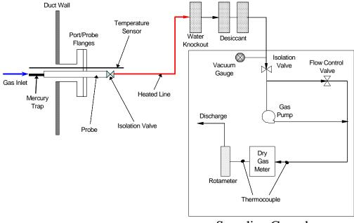
Figure K-1. Typical Sorbent Trap Monitoring System
