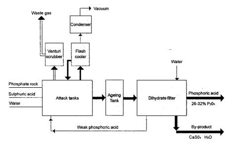
Within the attack tanks, an exothermic reaction occurs, meaning that heat is produced from the chemical reaction. The heat is removed via the flash evaporation of water in the flash cooler. This provides an opportunity within a phosphate fertilizer plant for cogeneration, since steam is created which is otherwise wasted to the atmosphere via a condenser.
