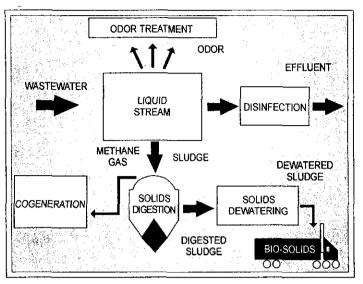
erators to produce electricity. The engines can usually run on digester or natural gas and supply electrical power to essential pieces of treatment plant equipment as well as the potential to feed the grid.
