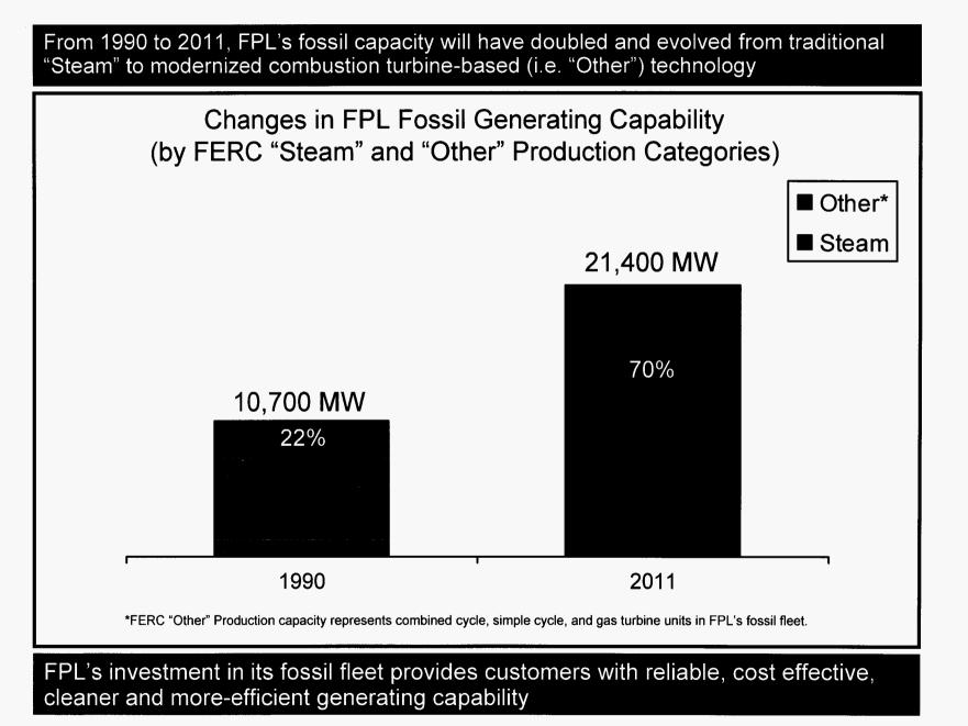
Docket No. 080677-E1 Changes in FPL Fossil Generating Capability Exhibit GKH-1, Page 1 of 1 FPL's fossil heat rate, reflecting fuel consumption efficiency, has improved nearly 19% since 1990 and is significantly better than the fossil industry average
