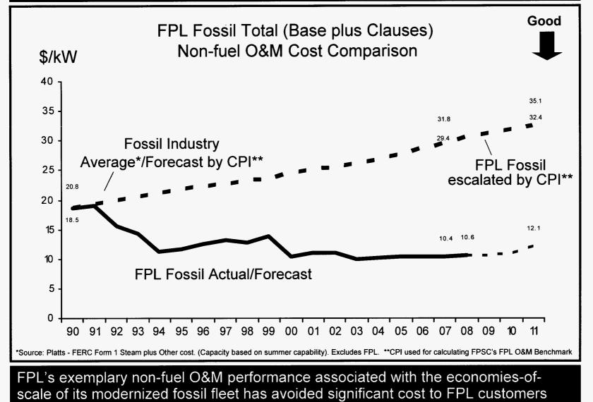
Docket No. 080677-E1 FPL Fossil Total Non-Fuel O&M Cost Comparison Exhibit GKH-8, Page 1 of FPL's fossil "Steam" plus "Other" base non-fuel O&M cost per kW of capacity is projected to be consistent with CPI inflation throughout the 2006-2011 timeframe
