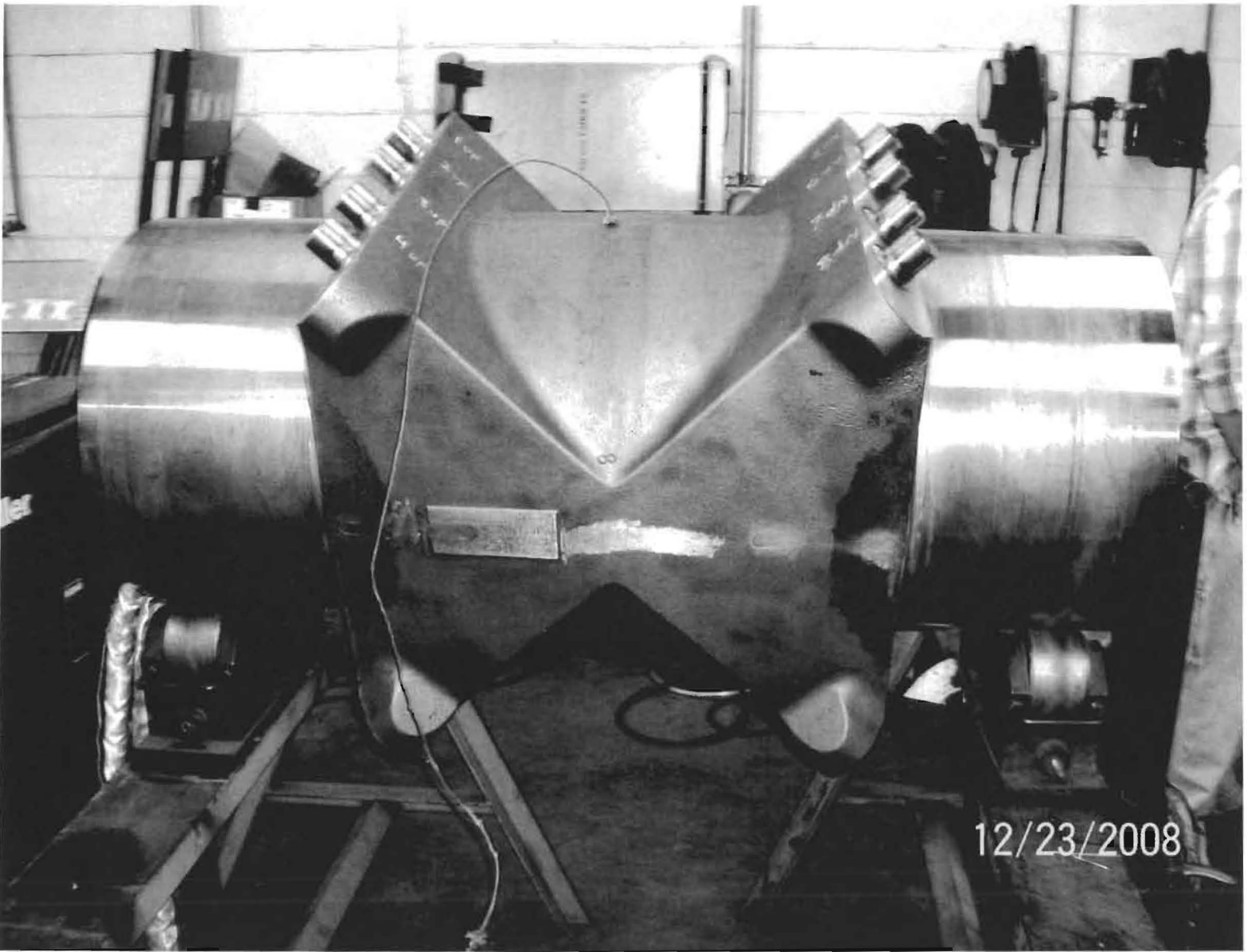
Docket No. 090009-E1 Ultrasonic Flow Metering Hydrostatic Pressure Testing of the System Exhibit RSK-3, Page 1 of 1
