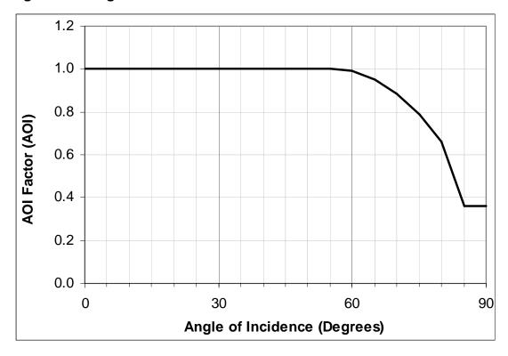
Figure 5-1: Angle of Incidence Factor
