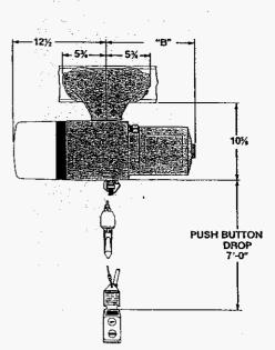
NOTE: TROLLEY WILL ADJUST FROM 5"x 10# TO 12"x 31.8# AMERICAN STD. I-BEAMS DIM. SHOWN ARE FOR MIN. SIZE I-BEAM WHEEL TREAD DIA.-4 WHEEL BASE-5½ MIN. RADIUS CURVE-2'6'
