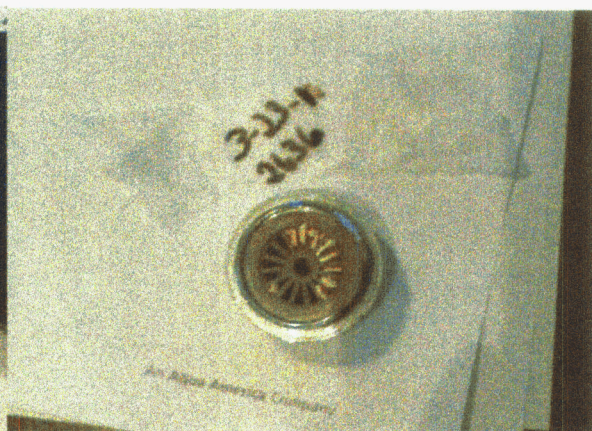
Example of sediment that gets stuck in aerators
