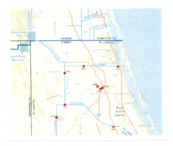
A conceptual plan has been developed for the proposed project that calls for the construction of a 3,200 acre reservoir and a 2,000 acre STA on land owned by Grove Land Utilities. The reservoir would provide eight feet of above ground water storage. Its footprint would be surrounded by a half mile strip of land also owned by Grove Land Utilities to avoid adverse impacts to adjacent land owners.
