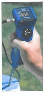
100 to 2,000 Hz Bandwidth: Filters: 3 Filter types: notch **Output indicators** Audio: stereo headphones Visual: 2-digit digital display Battery test: automatic 2 AA batteries (included) Battery type: Battery life: 24 hours minimum 0.66 lbs Weight (amplifier/display): 8.15"W x 3.3"H x 2.4"D Dimensions (amplifier/display):
