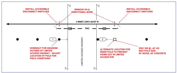
Fig 1. Limited Access Highway Crossing Schematic (Preferred)
