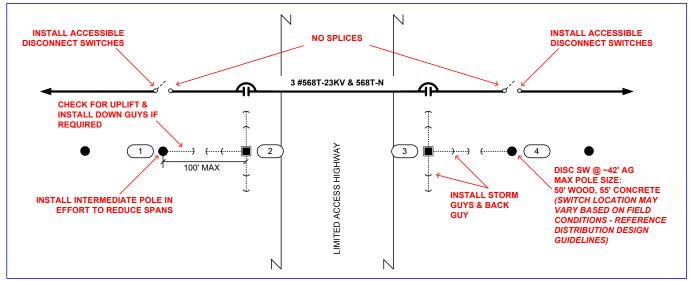
Fig 2. Limited Access Highway Crossing Schematic (Alternate)
