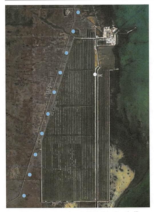
Figure 19. Configuration of extraction wells (blue dots) for Alternative 3D
