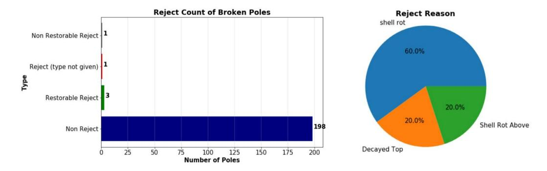
• After reviewing pole inspection data for the 203 broken poles, only 1 pole was not replaced prior to Hurricane Michael. This pole was scheduled to be replaced in January 2019.
