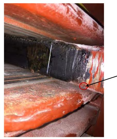
Discharge site to ground – Stator Core Finger Plate
