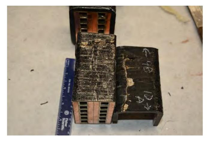
Separated insulation from ICP layer – Forensic process evaluating specimen for failure mode – none NOTED AT THIS TIME
