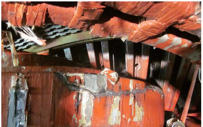
Failure mode identical to St. Lucie Unit 1 – tracking from insulation opening to ground over stator bar insulation
