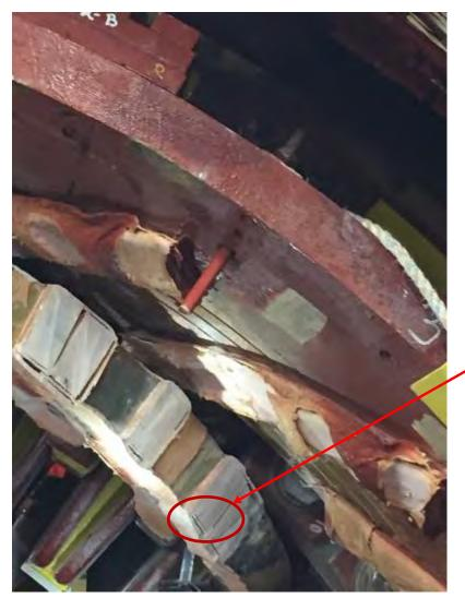
Extraction of Bottom Bar 17 - Fault location under blocking Hidden from view by blocking
