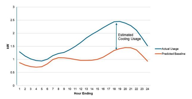
Figure 9: Methodology for Estimating Cooling Loads
