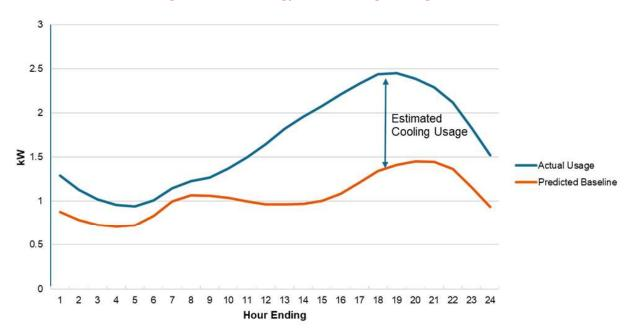
Figure 9: Methodology for Estimating Cooling Loads
