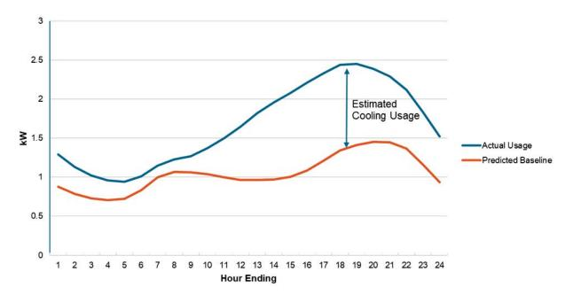
Figure 9: Methodology for Estimating Cooling Loads
