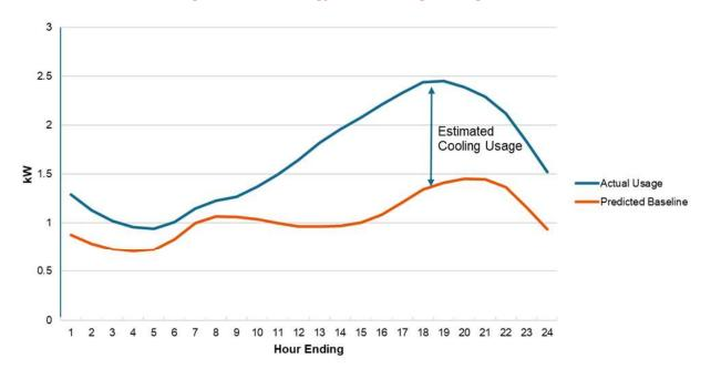
Figure 9: Methodology for Estimating Cooling Loads
