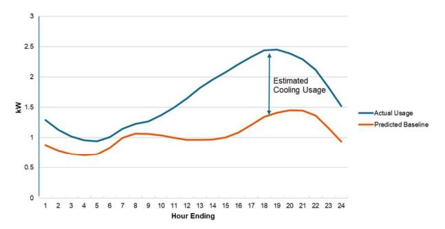
Figure 7: Methodology for Estimating Cooling Loads
