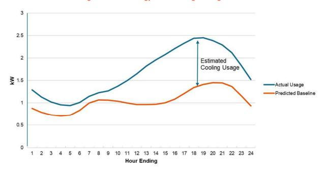
Figure 9: Methodology for Estimating Cooling Loads
