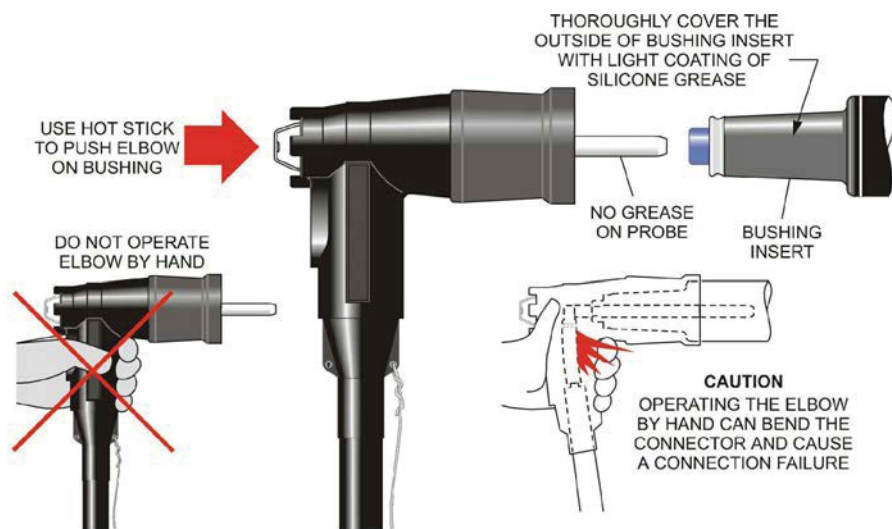
FIGURE 8 PUSHING ELBOW ONTO BUSHING USING HOT STICK
