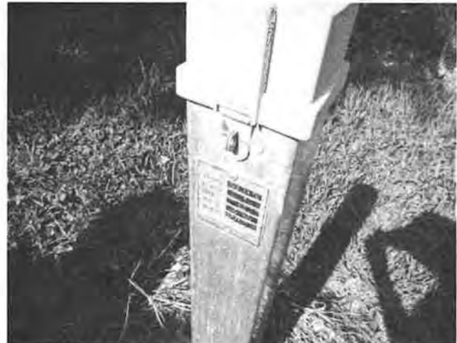
16. Unlocked monitoring well
