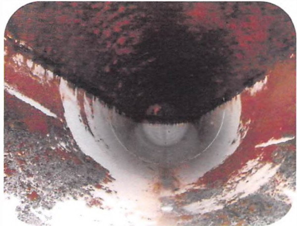
10. Internal After Cleaning Showing Coating Failure with Corrosion Throughout
