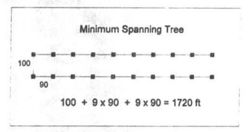
The Minimum Spanning Tree by necessity runs the full block length through the houses on both sides of the street. In this case, when we construct the distribution and drop configuration we find that it is longer, not shorter, than the Minimum Spanning Tree. The Minimum Spanning Tree is, to be exact, 5% shorter than the configuration AT&T and MCI cite.
