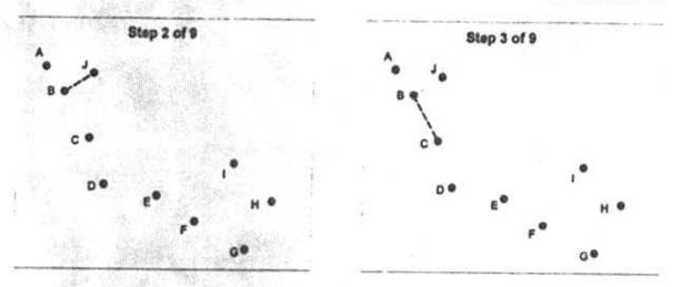
From A, B, and J, the shortest connection to any other point is from B to C. So we'll connect them, as seen on the right, above.
