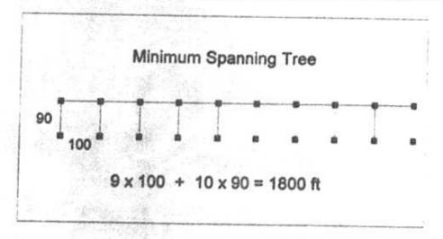
Now, if a single cable is run down one side (or the middle) of the street, and drops are extended to each house, the following configuration results. In this case, the DRD is identical to that for the Minimum Spanning Tree.
