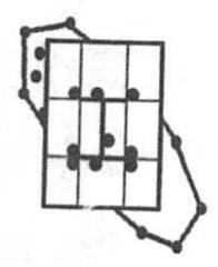
HAI 5.0a subtracts off two lot depths from the cluster North-South length to determine the length of the backbone cable. It also subtracts off two lot widths from the East-West cluster length to determine the length of the branch cable. In the figure shown above, there are two branch cables. Backbone and branch cable is laid in only the middle lot. A drop serves the house in each lot.
