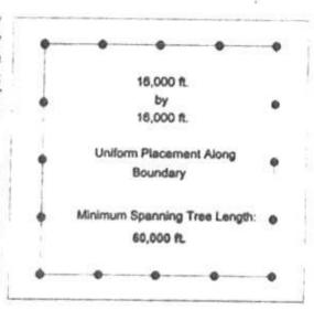
this uniform placement within the square (but, of course, every configuration of Minimum Spanning Tree for that placement of points has exactly the same length). Surprisingly or not, it is again 60,000 ft.
