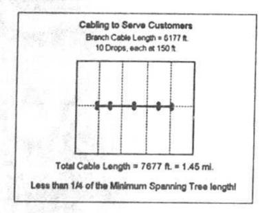
But note how closely the customers are squeezed toward the branch cable. The arrangement is unrealistic, both from the standpoint of cable length and from the standpoint of area served.
