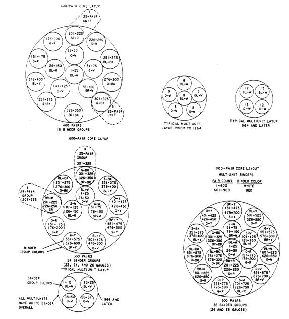
Fig. 11—Layup of 400-, 600-, and 900-Pair Even-Count BH and BK PIC Cables
