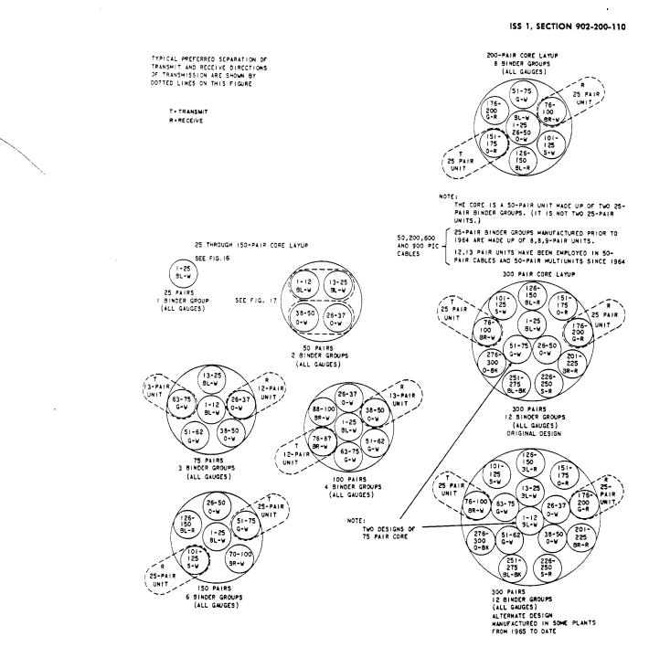
Fig. 10—Layup of 25- to 300-Pair Even-Count BH- and BK-Type PIC Cables
