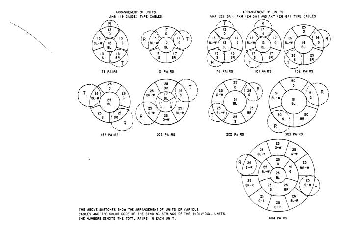
Fig. 15-Layup of 76- to 404-Pair AH- or AK-Type Odd-Count PIC Cables
