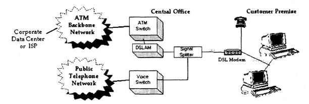
Figure 3 Typical configuration of a DSL system
