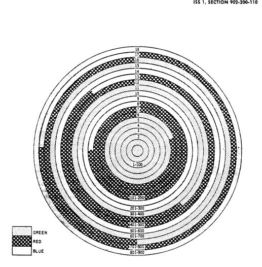
Fig. 18—Configuration of 900-Pair Layer—22 Gauge
