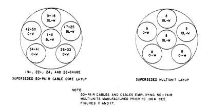
Fig. 13—Layup of 50-Pair and BH- and BK-Type PIC Cables and Multiunits
