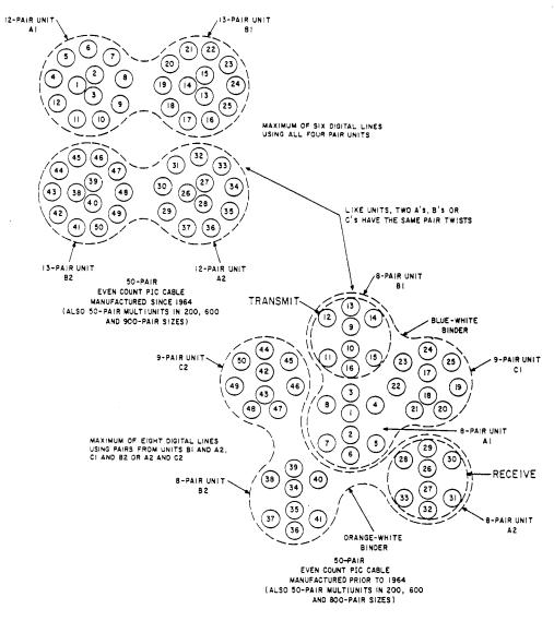
Fig. 17—Layup of 50-Pair Cable and 50-Pair Multiunits in Even-Count PIC Cable
