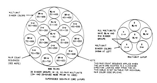
Fig. 12—Layup of BH- and BK-Type PIC Cables
