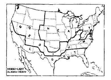
Fig. 250-1 Ceneral Loading Map of United States with Respect to Loading of Overhead Lines
