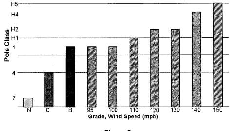
Figure 2 Required Distribution Pole Class vs. Typical Grade C Strength Requirements (NESC-2002)
