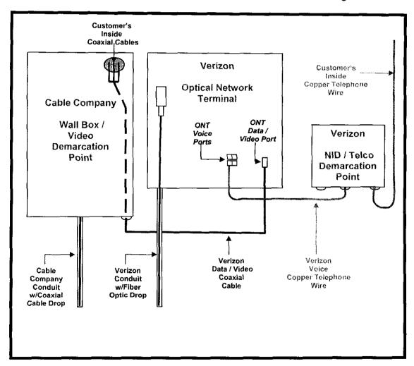
The diagram shows the cable company's conduit with coaxial cable drop, which previously (before Verizon won the customer) connected the cable company's pedestal (not shown) to the customer's inside coaxial cables at the video demarcation point in the wall box. When in operation, the cable company's coaxial cable drop can carry unregulated VoIP, broadband and cable services.
