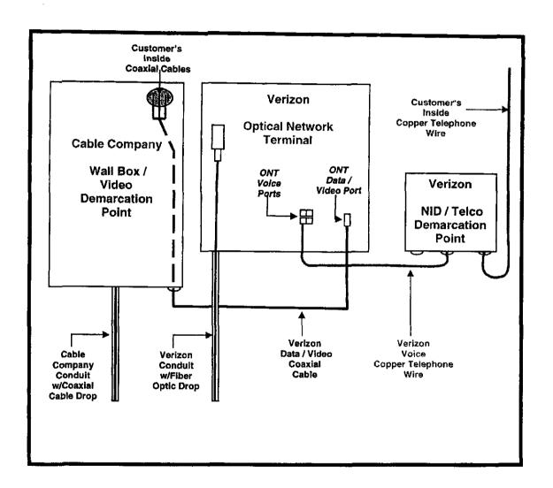
6. The diagram shows the cable company's conduit with coaxial cable drop, which previously (before Verizon won the customer) connected the cable company's pedestal (not shown) to the customer's inside coaxial cables at the video demarcation
