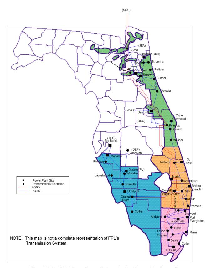
Figure I.A.2: FPL Substation and Transmission System Configuration
