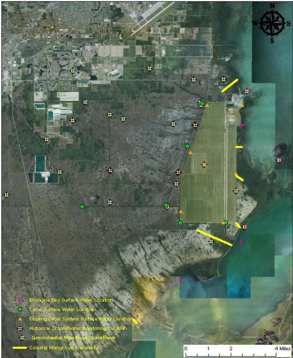
**Figure 6. FPL Turkey Point Power Plant Groundwater, Surface Water, and Porewater Monitoring Locations**
