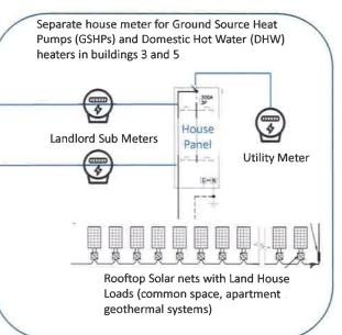
Electrical for GSHP's and DHW heaters on buildings 3 and 5 connected to landlord house meters
