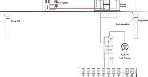
Rooftop solar to offset Geothermal District loads (Geo pumps and Well Pumps) Separate landlord house meters in 2 energy centers
