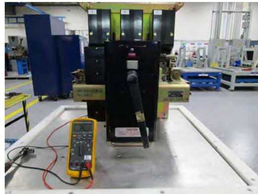
Breaker Closed, Switch Contact Open
