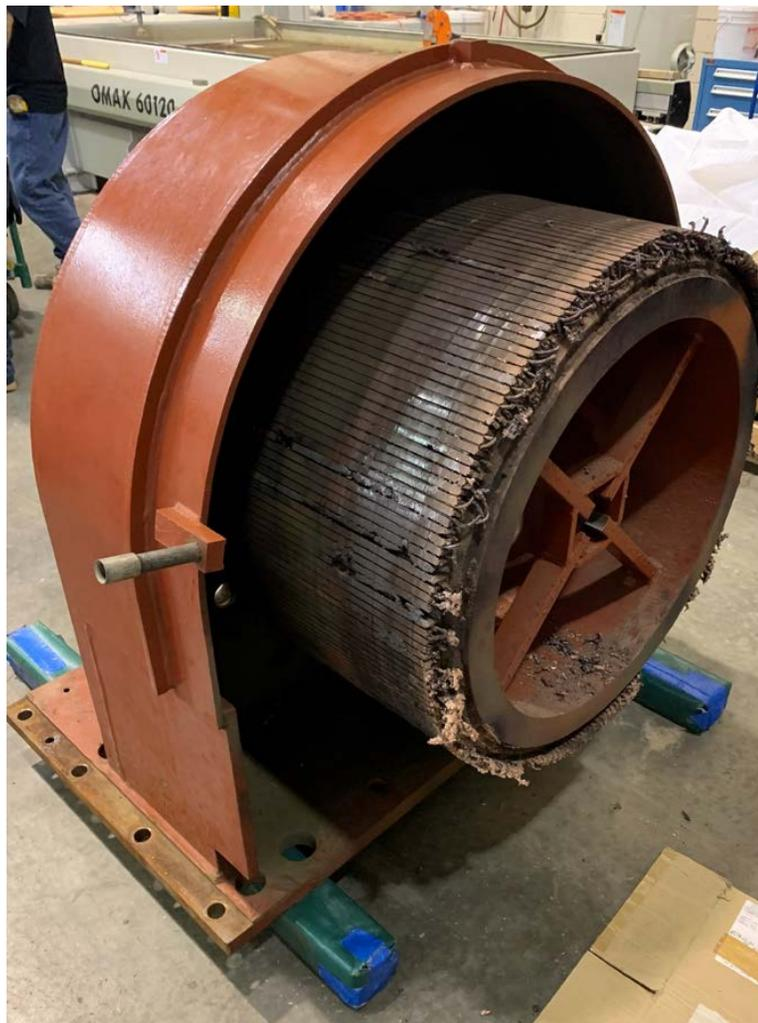
Fig. 5 U4 PMG Stator Removed
