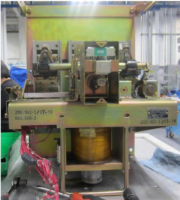
Breaker with the Auxiliary Switches and Control Relay Removed
