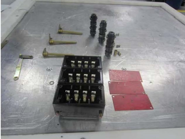
Disassembled Auxiliary Switches No issues were found with the auxiliary switch assembly.
