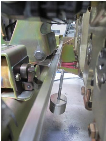
Additional Weight Added to the Operating Mechanism Trip Bar
