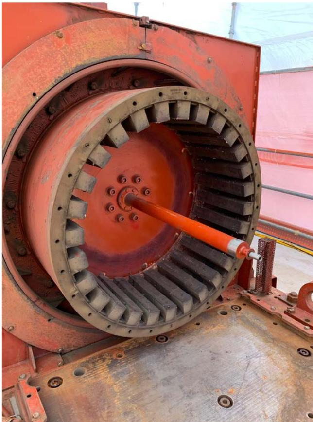
Fig. 8 PMG Pole Support w/ Magnets
