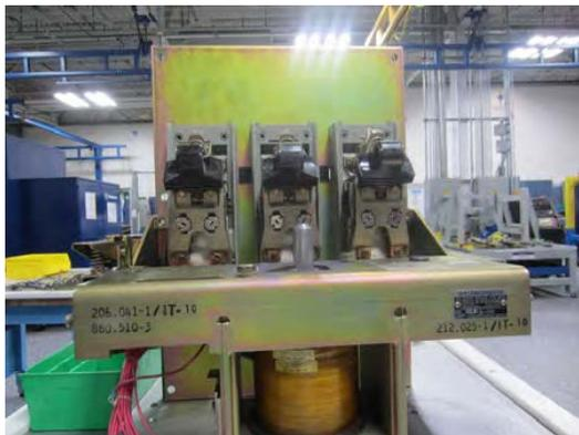
Breaker with the Operating Mechanism Removed
