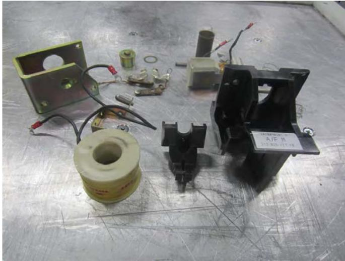
Disassembled Control Relay No issues were found with the control relay assembly.
