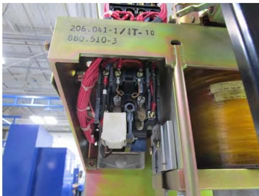
Control Relay with Front Cover Removed
