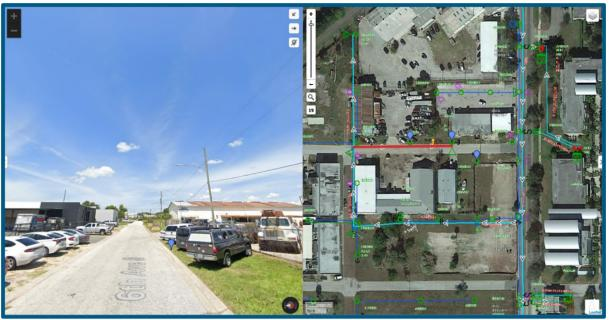
Figure 3: The teal tap line branches cjf the main road through an open lot to side streets where it splits again. It serves a few customers with minimal, to no vegetation. The street view is a view of the red line where there are no vegetation concerns.
