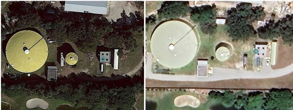
Aerial view of the Aquarina water system at acquisition (left) and currently (right). Note recoated tanks, cleared vegetation and debris, new access roads, and temporary hydro-pneumatic tank on site.
