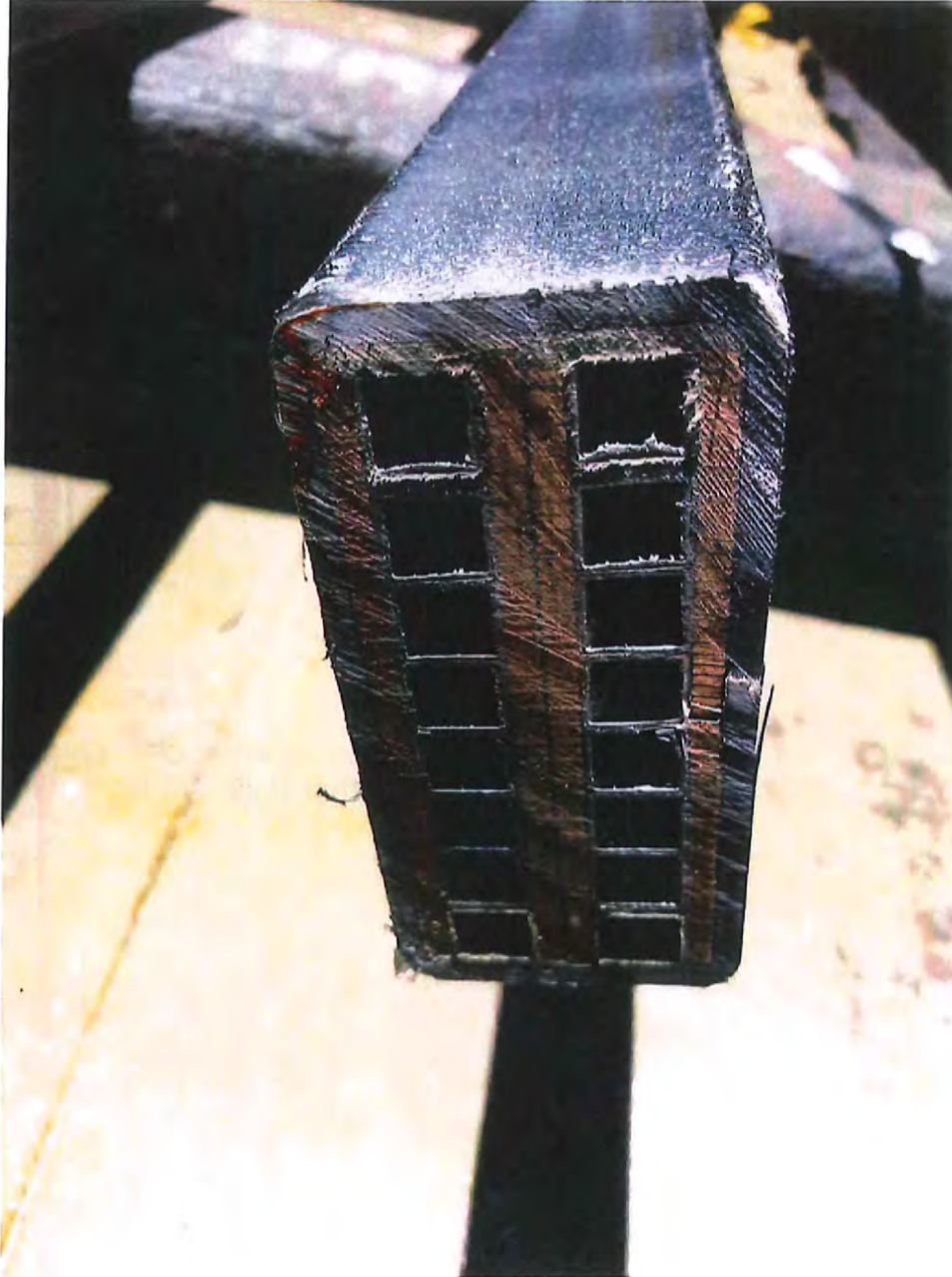
Figure 6 – Section of Stator Bar Removed from Unit 1 Generator 2019 Rewind
