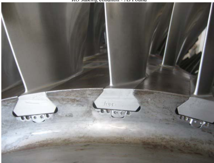
RO Biscuit Modification Completed in HSC
