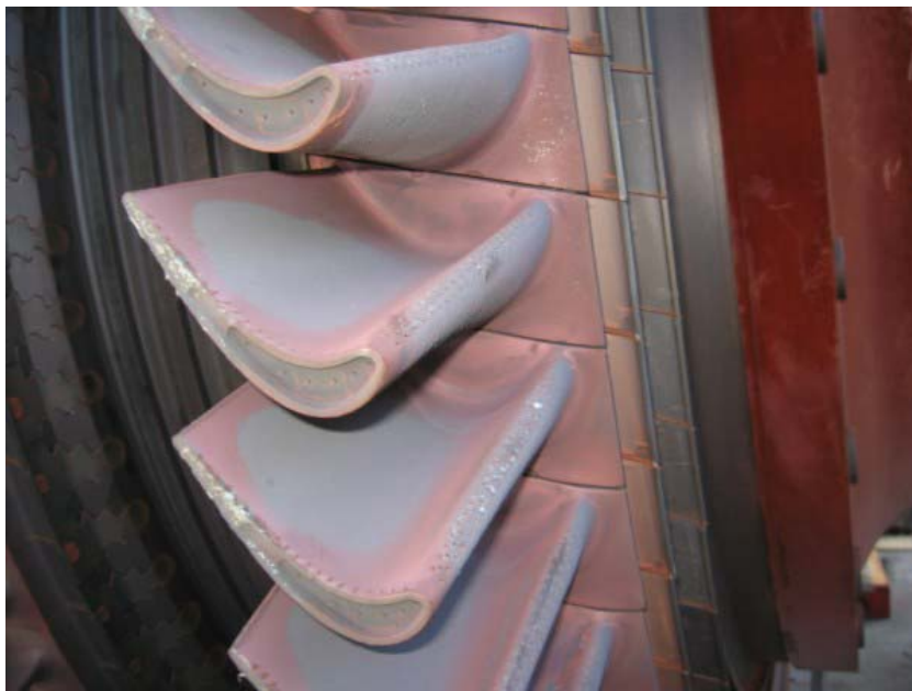
1st stage bucket - As Found Condition
