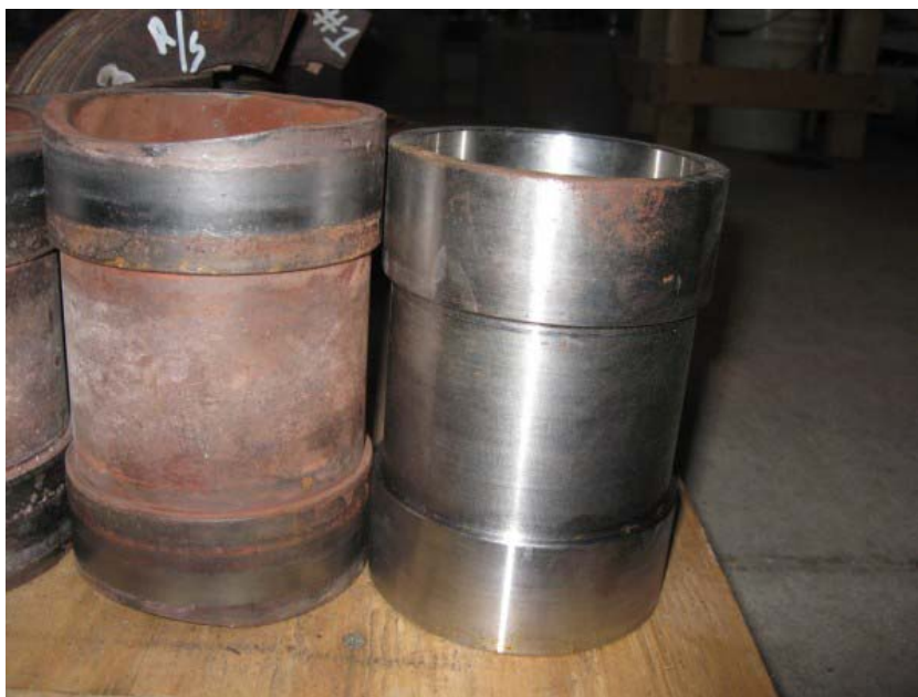
Outer crossfire tubes -- Note the different lengths
