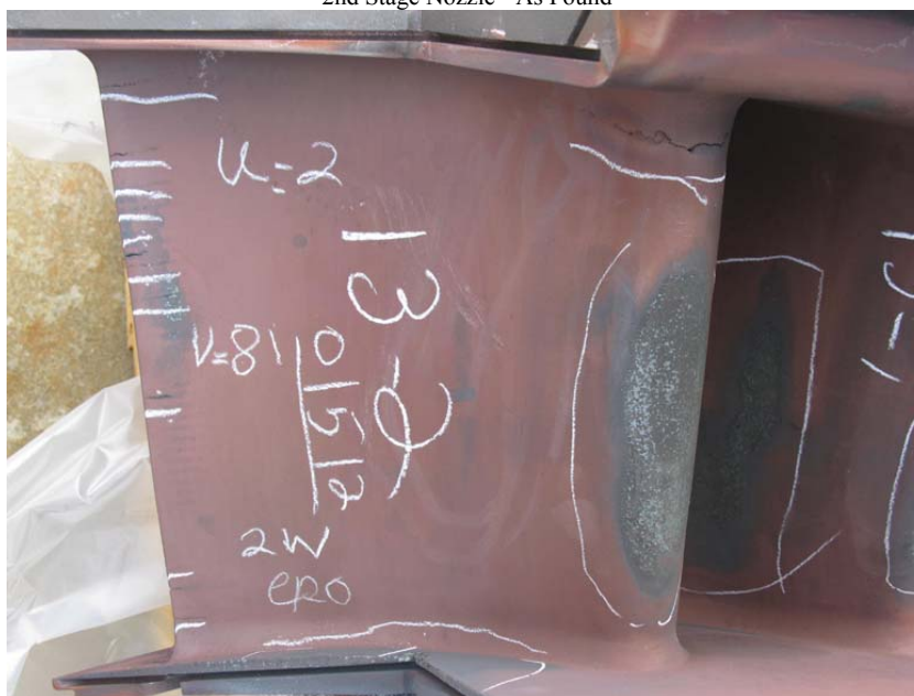
2nd Stage Nozzle - Typical Cracking
