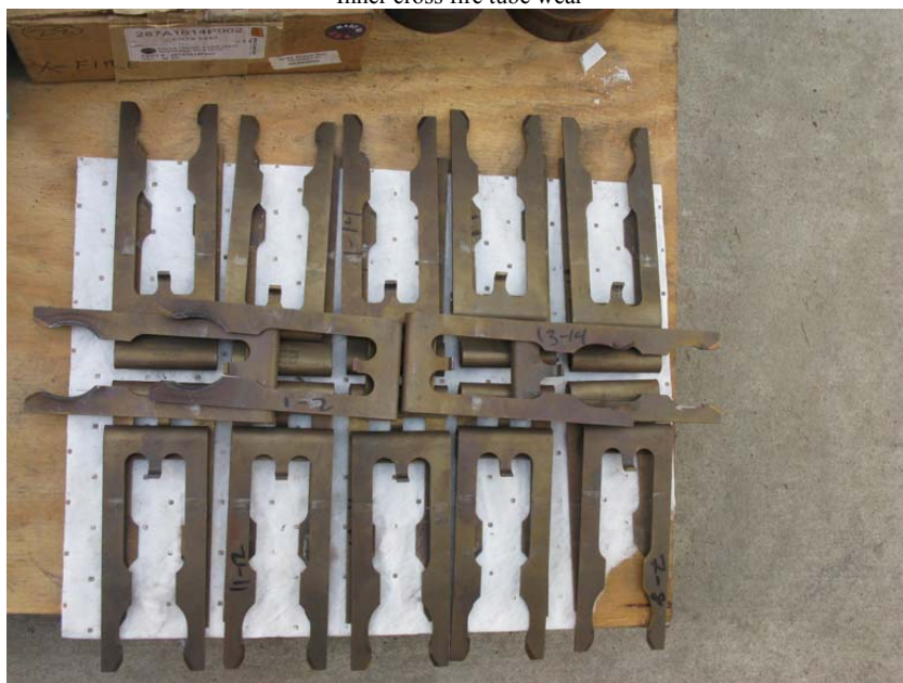
Retaining clips as found
