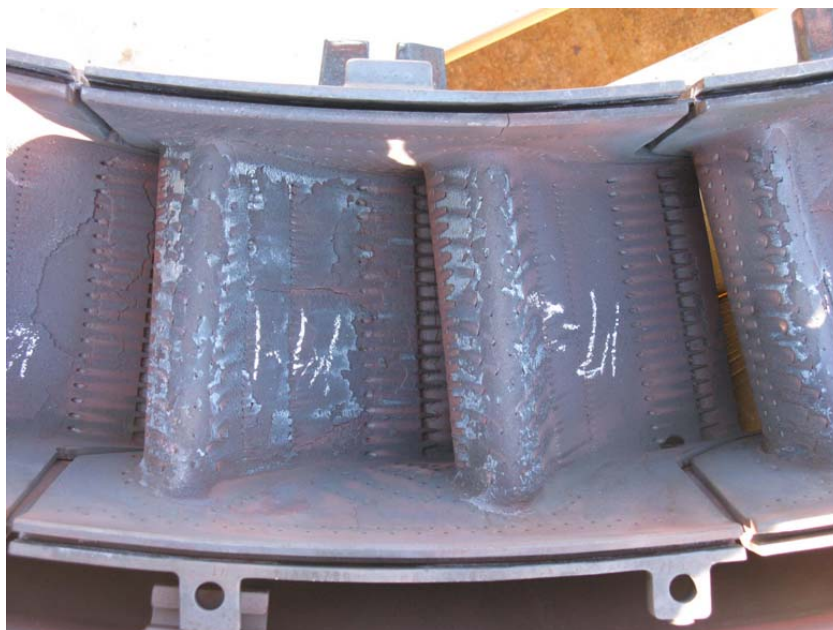
1st stage nozzle - As Found Condition
