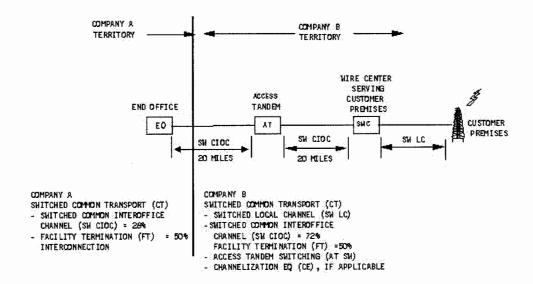
Assume 20 miles of Switched Common Transport (CT); 20 miles of Switched Dedicated Transport (DT); and 8,000 minutes of use. Further, assume a billing factor from NECA 4 of 28% for Company A and 72% for Company B.
