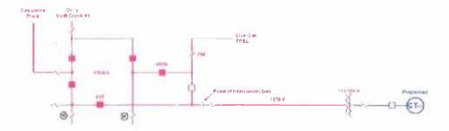
Point of interconnection requested for study by interconnection customer for the 230kV unit:
