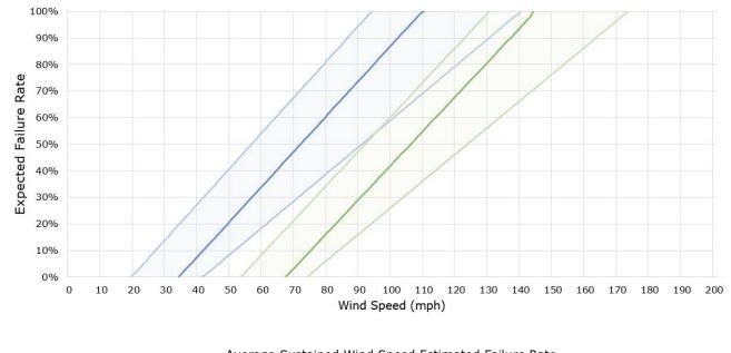
Average Sustained Wind Speed Estimated Failure Rate
