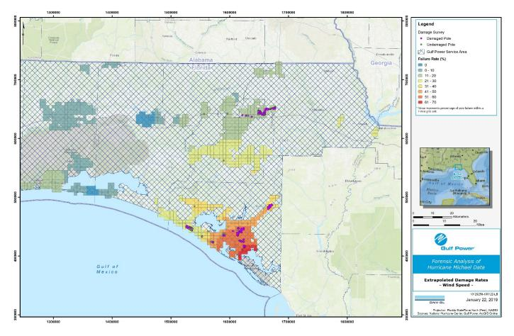
Figure 5-2 Extrapolated Gulf Power Damages to the Eastern District Service Area
