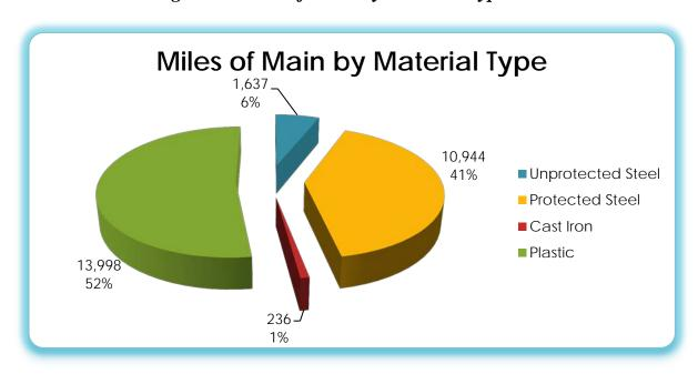
Figure 7 below shows the quantity and age of the existing pipeline in Florida as of December 31, 2012. The age of the cast iron and steel pipelines without corrosion control, range in age from 50 to 70 plus years, and account for 26 percent of the total pipeline in Florida. These aged and/or unprotected pipes have a significantly higher leakage rate than that of the newer plastic pipeline that was placed after 1971.
