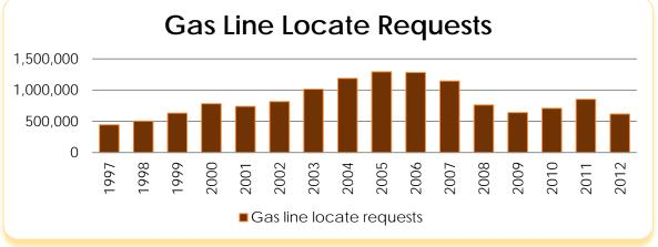
The number one cause of damage to natural gas pipelines in Florida, as well as the entire United States, is dig-ins (pipelines cut or damaged by others engaged in excavation activities or directional drilling). Underground utilities can sustain damages from just a small nick of the outer lining of the buried facilities, causing leaks, water intrusion, or corrosion.
