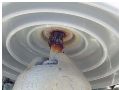
Typical State 4 “Ball & Socket” Insulators
